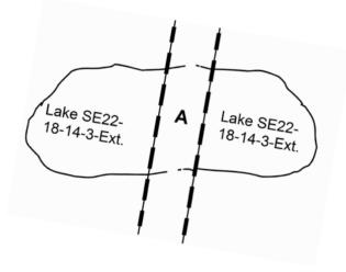
b) Where a road widening is adjacent to an original road allowance, the widening lines shall stop at the water bank and no area shall be taken within the water body on the widening. The original road allowance shall be one continuous parcel, not broken by the water body.
