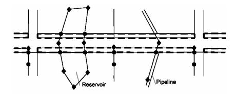
c) Where the new road right of way intersects two or more adjacent and parallel previously surveyed right of ways, only the intersection with one of the previously right of way shall be monumented. The monumenting the intersections with all previously surveyed right of way may be a safety issue.
