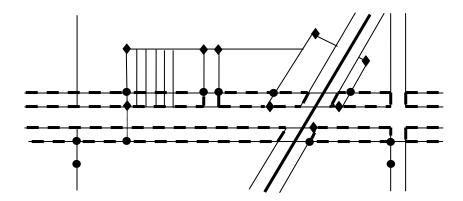
b) Where the new road right of way intersects a previously surveyed reservoir or drainage ditch where the entire perimeter has been monumented and a deflection exists on that survey within the new right of way, both limits of the new road right of way shall be monumented at the intersections. Intersections with all other registered plans shall be monumented as stated in Section 1 of this Part.
