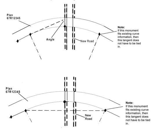
c) Where a simple curve ends at a line that is not tangent to the curve, the angle between that line and radius shall be shown.
