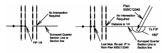
i. Where a road right of way is surveyed adjacent to a road allowance and begins or terminates at, or crosses a quarter section line that has not been previously surveyed, a monument shall be established on the surveyed limit at 90 degrees to the quarter section monument.
