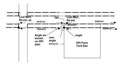
c) Where the unmonumented limit of the new survey intersects the DPI Farm Yard Site, a standard iron post shall be established on the limit of the new survey referencing the intersection point.
