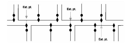
b) Where a surveyed road diversion exists along a road allowance and the intent is to abandon the road diversion, the monuments on the road diversion do not have to be located unless they are required for re-establishment purposes. A report should be included with the plan indicating that the road diversion will be abandoned.
