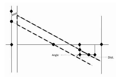
b) Where the unposted limit of a road right of way passes through a previously surveyed road right of way where the surveyed line is not coincident with the section/quarter line, the intersection of the production of the surveyed line and the monumented limit shall be monumented.
