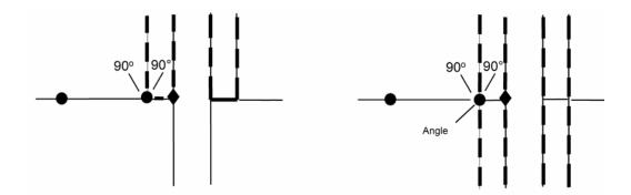
ii. Where a new road right of way is surveyed superseding an existing road right of way and begins or terminates at, or crosses a quarter section line that has not been previously surveyed, a monument shall be established on the surveyed limit at the intersection of the new road right of way limit and a line from the quarter section corner through the road right of way monument.
