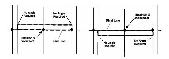
a) Where a road right of way is surveyed adjacent a quarter section line and one of the limits of the right of way is coincident with the quarter line, monuments may be established on the said right of way limit. The section lines at both ends of the new road right of way do not have to be tied in unless required for reestablishment purposes.
