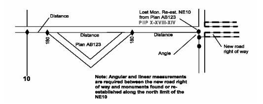
b) Where a new survey begins or terminates at a surveyed limit, an angular and linear measurement shall be secured between the surveys and shown on the plan.
