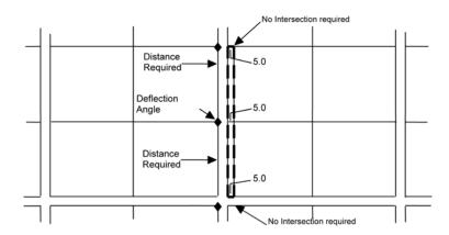
**NOTE:** Angular or linear ties are not required east or west of the road allowance unless required for re-establishment purposes.
