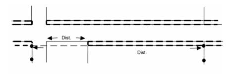
c) Where a parallel extra width or restriction occurs on the unposted limit of the road right of way, at minimum a single monument shall be established on the monumented limit opposite one end of the extra width or the restriction.
