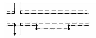
b) Where an extra width or restriction occurs on the monumented limit of a road right of way and the extra width or restriction is around a descriptive parcel (metes and bounds), monuments are not required at the intersections.
