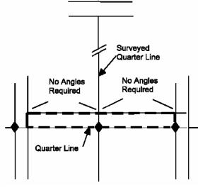
b) Where a road right of way is surveyed adjacent to a road allowance and the unsurveyed limit crosses a previously surveyed quarter section line, the surveyed quarter line is not required to be intersected. This also applies when the unsurveyed limit crosses a section line.
