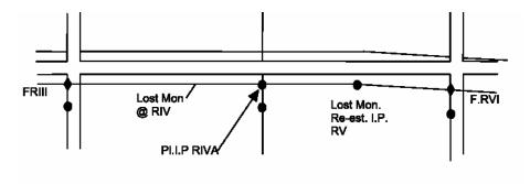
b) All secondary monuments marking the intersection of any subsequent surveys crossing the road right of way shall be found or re-established and connected to the survey.
