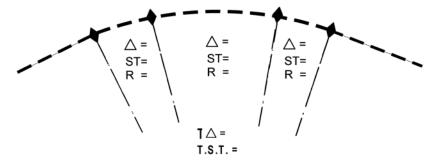
b) When intersecting an existing curve or when it is necessary to re-establish one end of a curve, a minimum of two curve monuments and one tangent shall be found or re-established to verify the existing curve information.
