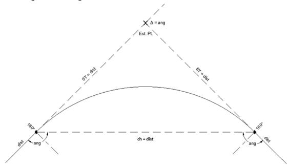
iii. The following five diagrams are acceptable options for intersecting a surveyed lined with a curve.
