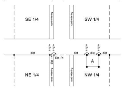
39. If it appears unclear as to how two boundaries are related, additional angular and linear measurements will be required to clearly demonstrate how the boundaries correlate to each other.
