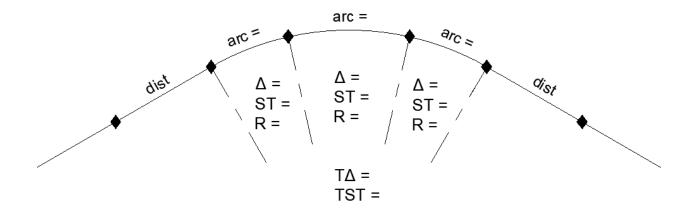
iii. Retracement of existing replacement curves based on formerly prescribed tables (Arc definition for roads and Chord definition for railways) must show three simple curves and include the Total Subtangent (TST) and Total Delta ( $T\Delta$ ).
