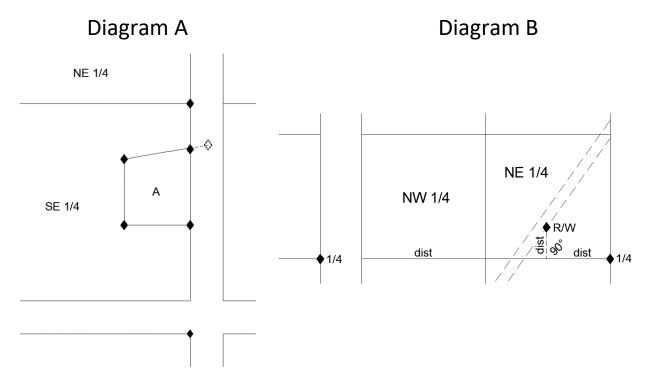
In diagram A, the monument found in the road allowance must be moved onto the section line using the bearing of the found monuments. This bearing governs the north limit of parcel A, but the monument in the road allowance does not govern in place, as it falls within the road allowance.
