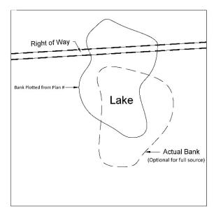
12. Where a Surface Lease (feature) Plan crosses a bank based on title, the titled bank is to be shown as a dashed line within the feature and the actual bank is to be defined and shown as a solid line. A small portion of the actual bank must be shown as a dashed line on both sides of the feature and is optional to be shown through the full source.
