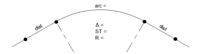
ii. Replacement of planned or constructed spiral curves must show three simple curves and include the total Deflection Angle  $(T\Delta)$  and total subtangent (TST).
