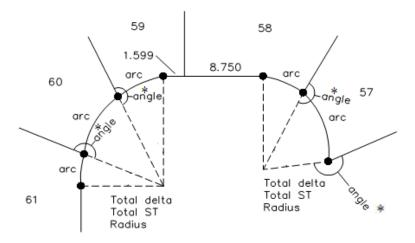
\* When the angle from lot line to radius is not 180° or when the angle from the subtangent to the radius is not 90°, the angles are to be shown.
